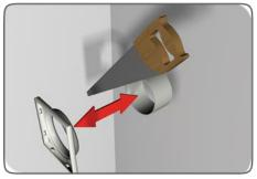
From the opposite end/ bottom of the Shower Drain Top mark the same distance as previously measured. Using a hard point saw, cut the excess from the bottom of the Shower Drain Top. It may be necessary to file or sand the cut edge to make it completely flat.
