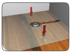
Replace the flooring ensuring that an adequate hole has been cut to allow for the shower drain to be exposed through the floor. Please note: The hole size should be no bigger than 180 x 180mm.
