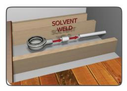
For water to drain away properly, the wastepipe must have a fall of at least 3cm per metre. The wastepipe must be properly supported to hold its own weight and that of the shower drain. Connect the Shower Drain to your wastepipe using a 2" solvent weld connector (also supplied is a shower drain reducer if required). Once the solvent weld has set; pour water down the drain to check that the waste is not blocked and that there are no leaks.
