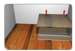
Remove flooring as necessary to carry out works to the wastepipe. Please note that if there is a joist in the way of the Shower Tray you will need to consult a professional joiner or structural engineer for advice.
