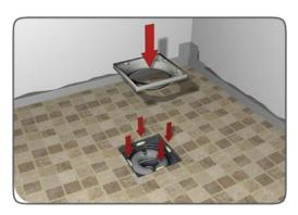
Place a small blob of tile adhesive in the middle of all four sides of the Shower Drain Hole in the Shower Tray. Gently ease the Shower Drain Top into position in the Shower Tray. Leave to set for approximately 3 to 5 hours. Fill the gap between the edges of the Shower Drain Top and the start of the tiles with the same grout used during tiling OR a colour match silicone sealant. Place the Shower Drain Finishing Grate into position.
